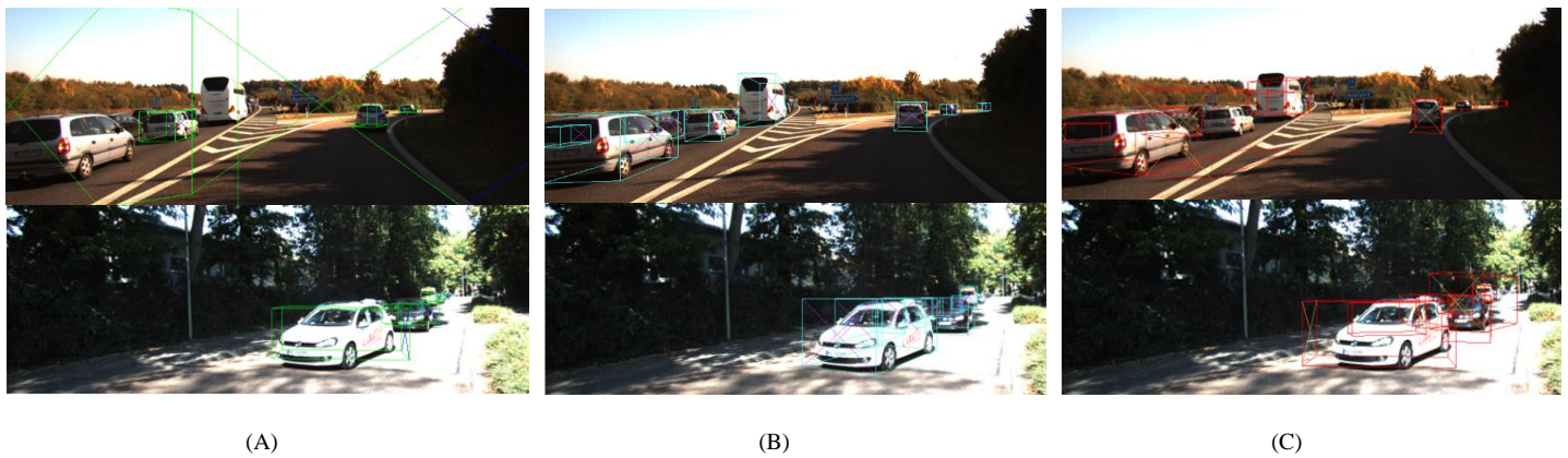
Figure 1: Comparison between the three methods for object detection in two testing images – the 007475.png (top three panels) and the 007479.png (bottom three panels). (A) Deep Learning & Geometry: 4 car objects detected in top image (007475.png) and 4 car objects detected in bottom image (007479.png). (B) Triangulation Learning Network: 7 car objects & 1 bus object detected (top) and 6 car objects & 1 bus object detected (bottom). Monocular 3D Object Detection: 7 car objects & 1 bus object detected (top) and 6 car objects & 1 bus object detected (bottom).
