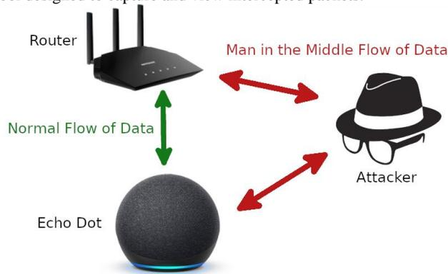
**Figure 1.** Diagram of a Man-in-the-Middle attack, showing how data moves comes and goes to the Echo Dot. During the attack data is sent to the attacking computer and then the router rather than directly to the router. This passive attack allows for data to be collected on the encryption method used to protect the data coming to and being sent from the Echo Dot. That knowledge could give the attacker information on how to further attack the Echo Dot.
