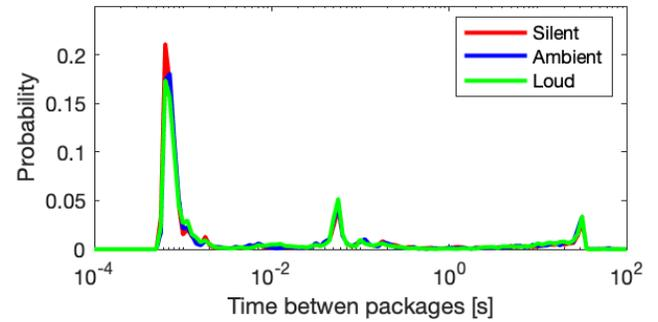
**Figure 2.** Histogram displaying the time between packets to the probability of that time. The tested sound variables were laid on top of each other to better visually compare the variables. The scaling used for the X axis was chosen because of the data's wide range of values. This histogram presents that no matter how much activity is within a room it will be just as easy for an attacker to listen in on its occupants.
