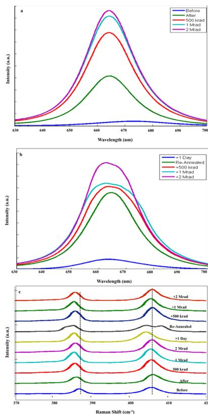
**Figure 3.** PL and Raman spectra of MoS<sub>2</sub> irradiated with X-rays, over two sets of exposures. PL spectra of (a) the first set and (b) the second set. (c) Raman of both sets of exposures. Each set consisted of taking the as-is (or for second set, 'rested') flake, vacuum annealing the sample, and then exposing it to increasing doses of radiation.
