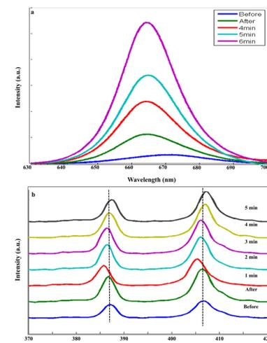
**Figure 2.** (a) PL and (b) Raman spectra of MoS<sub>2</sub> exposed to ozone plasma for various time points.
