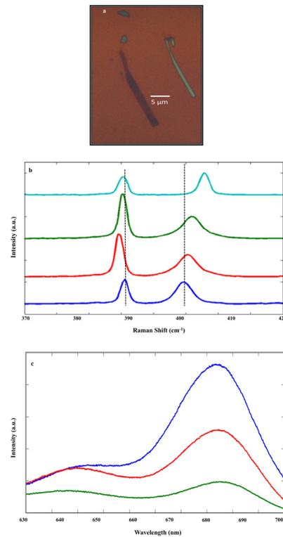
**Figure 1.** (a) A MoS<sub>2</sub> flake with varying thicknesses, where the translucent purple indicates a monolayer region. (b) Raman and (c) PL spectra of MoS<sub>2</sub> flakes of varying thicknesses. The spectra show monolayer (blue), bilayer (red), tri-layer (green) and bulk (cyan).
