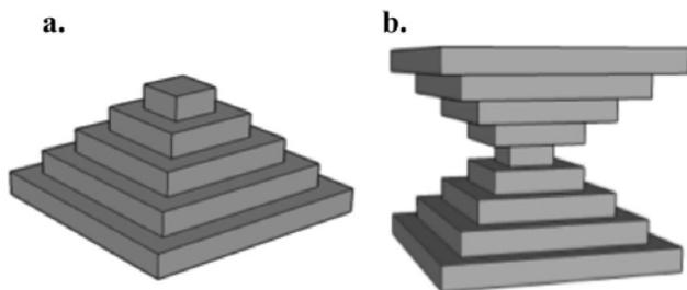
**Figure 3.** Rendering of plans for future three-dimensional structures: **a)** A pyramid consisting of stacked squares will demonstrate the system’s ability to create structures with variations in all three dimensions. **b)** An hourglass consisting of two stacked pyramids, one inverted on top of the other, will demonstrate the ability to produce more complex structures.
